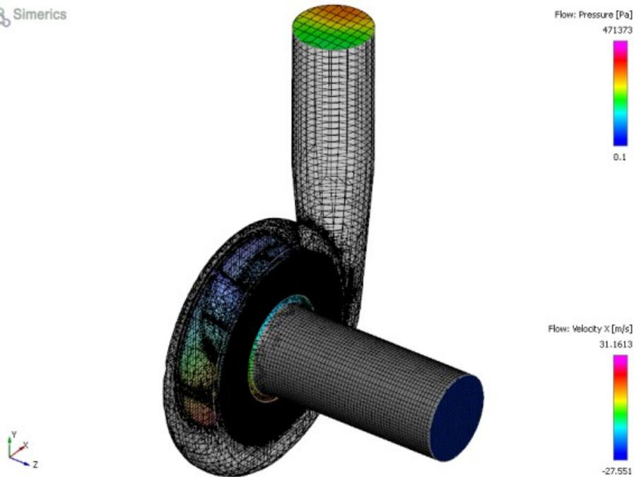
**Figure 6. An illustration of the output of the pressure and velocity field from SimericsMP**
