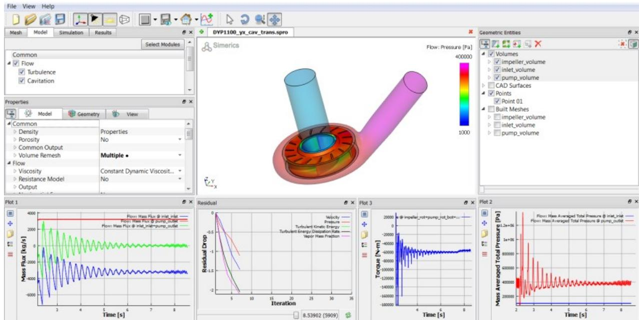
**Figure 4. CFD model of Dredge 1100 (surface pressures and x-y data plots)**
