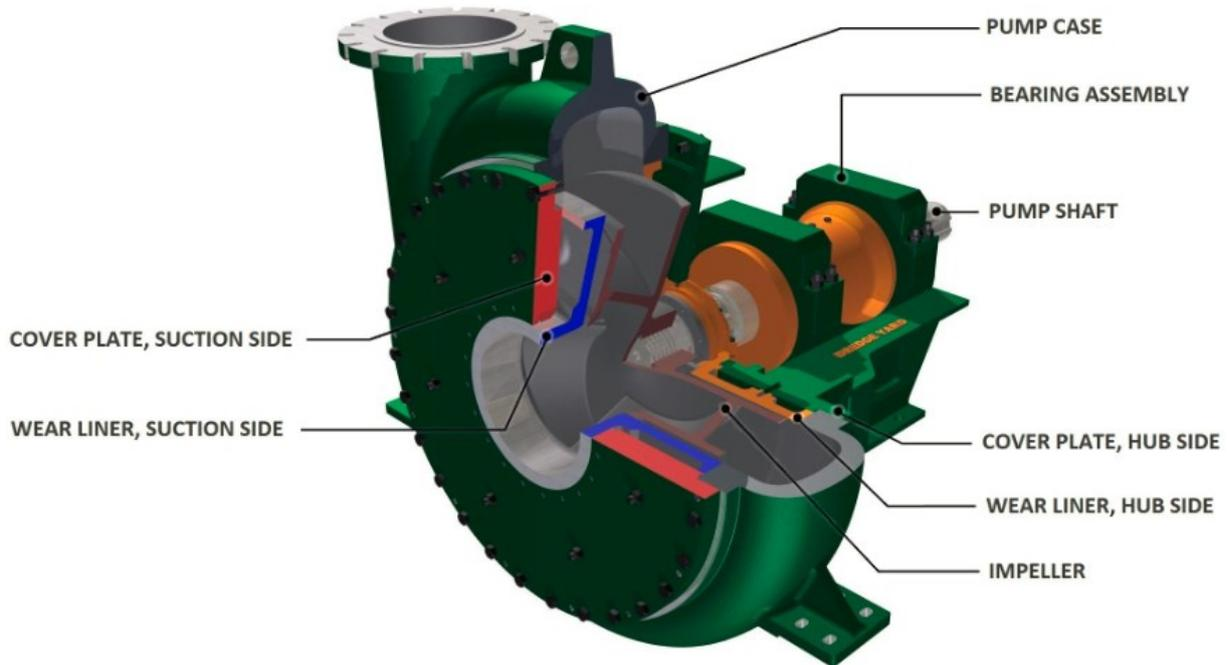
**Figure 2. A sectional view of the dredge pump**
